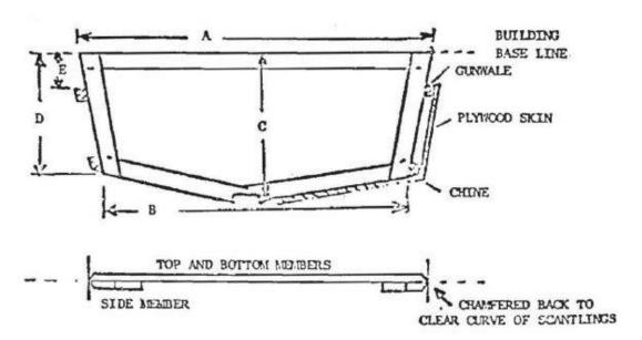
Note: It will be seen that the plywood is in contact with the moulding frames at the bottom but not the sides.
